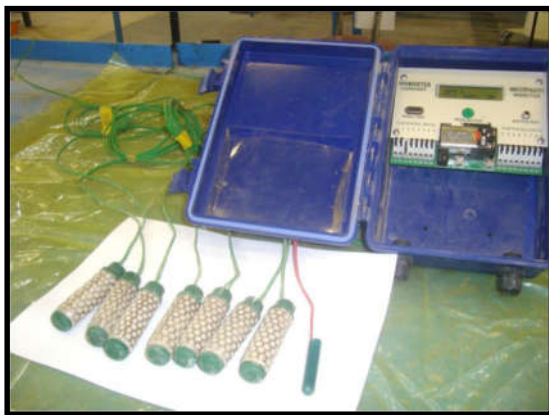
Figure 5. Suction monitor 900M with soil and temperature probes.
