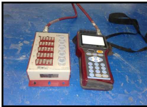
Figure 3. Data logger connected to five channel switching box.
