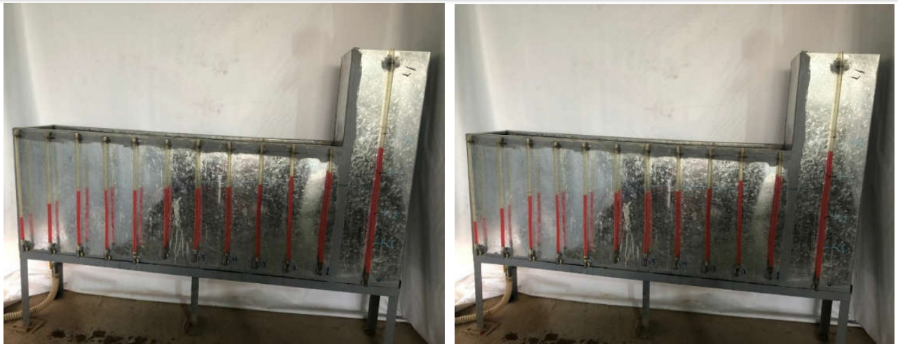
Figure 3. Phreatic line measurements.
