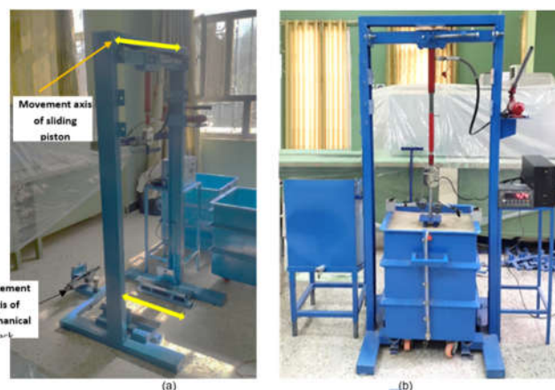
Figure 3. Manufactured testing equipment: a) Sliding piston and manual jack, b) Setup of test.
